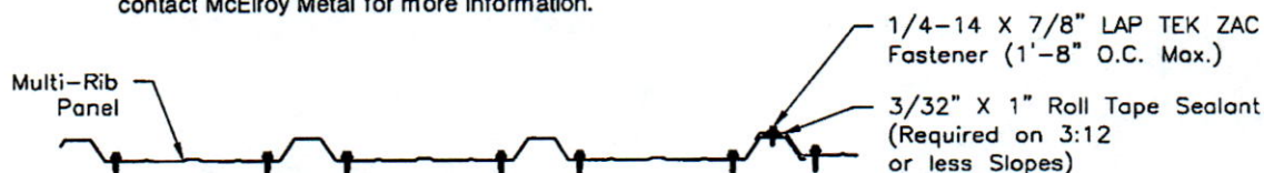
FASTENER PATTERN (@ Eaves, Ridges & Endlaps)
